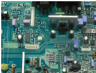
Digital Amplifier main circuit. SMD components.
